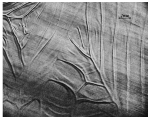
Fig. 4. Stripes at 43.5 hr. A set of five parallel stripes is located on the right side of the photo. Initial acid concentration = 7.4%.
