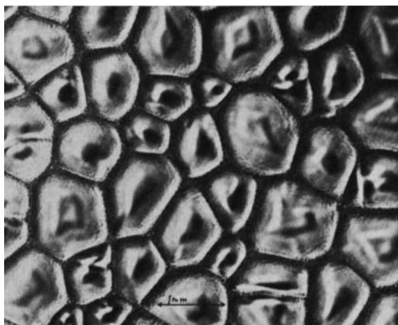
Fig. 2. Stationary cells 12 min. after formation of the interface. The lower phase contained initially 10 wt.% acetic acid in glycol. The upper phase is ethyl acetate.
